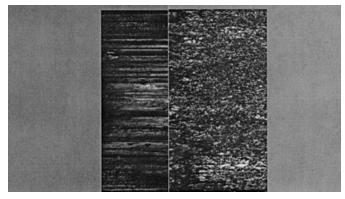
FIG. 6—IBIS comparison image of reference sample (B2) copper-jacketed bullet and known match (B3) lead bullet.
