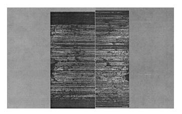
FIG. 1—IBIS comparison image of reference sample (E1) and known match (E2) copper-jacketed bullets.
